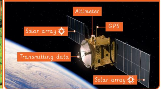
Weather satellites collect and send data back down to Earth, after monitoring the atmosphere from space.
